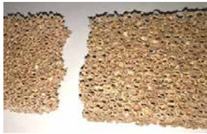
Combustor Problem - Broken Combustor
